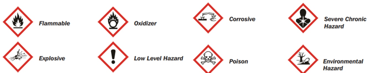
Figure 1.4: Internationally accepted safety symbols. credit: Globally Harmonized System of Classification and Labeling of Chemicals, United Nations New York and Geneva, 2005
